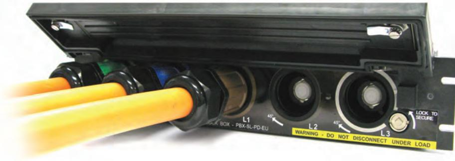
A PowerLock Box is a 3 phase high power connecting unit, used as a termination point for power cables. The boxes include a number of safety features to prevent incorrect connection and disconnection. All PowerLock devices are 'keyed' to eliminate the possibility of connecting with the wrong line, and color coded to suit international 3 phase standards.
