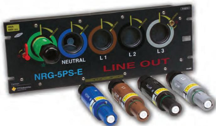
The NRG Sequential mating box comes in a 19" rack format and guarantees the proper sequence of mating and un-mating a set of PowerLock connectors. All ports are keyed to ensure that only the correct connector is fitted.
