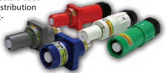
PowerLock connectors are easy to terminate to cable using either industry standard crimp tools or set-screw contacts. The silver plated contacts are available in 2 continuous current ranges, those with brass contacts are suitable for use up to 400 amps and those with copper contacts up to 660 amps.
