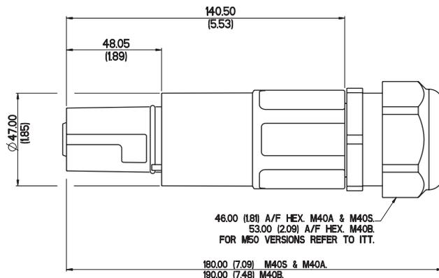
Line Drain is the connector with a female contact which is not normally the live part, however they are fitted with a spring loaded plastic cap that prevents accidental finger touching of the contact, and the connector meets IP2X requirements. Contacts are available to suit cable conductors from 25mm<sup>2</sup> to 300mm<sup>2</sup>.
