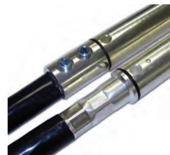
Cable glands meeting IP67 requirements are fitted to the connectors, 4 sizes are available that cover a range of cables with outside diameters from 15mm to 38mm. When selecting the M50 gland, please note that this is supplied with an adaptor (not shown above) that steps the connector up from M40 to M50.
