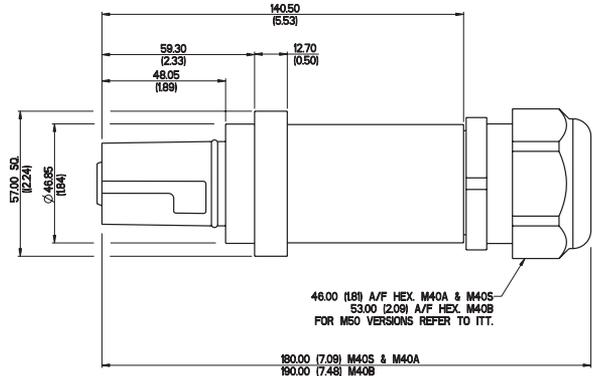
Panel Drain connectors (SKPP) can be supplied with a backshell to provide a watertight fitting to the cable. These connectors are supplied with a loose female contact that is fitted to the cable before being assembled into the connector housing.
