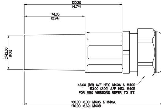
Line Source is the connector with a male contact which is normally connected to the source of the power. The contacts are fitted with a plastic end cap that prevents accidental finger touching of live parts of the connector and meets IP2X requirements. Different contacts are available to suit cable conductors from 25 mm<sup>2</sup> to 300 mm<sup>2</sup>.
